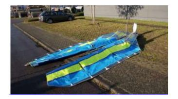
Push the rear sections of the leading edge tubes from the rear into the sail. Let the swivel tip exit the double sail at the zipper opening and push the tube into the front leading edge tube with the swivel tip cable pointing up. The swivel tip will swing to the rear. Press both snaps in and see that both snap out again through the holes in the front tube.
