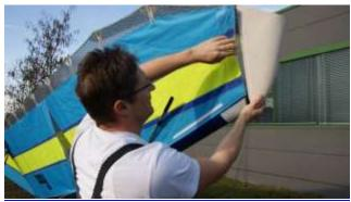
Fit the two sail end caps [winglets] outside, exactly at the front of the sail and close the Velcro at the edge of the upper sail first and then the one at the edge of the lower sail.
