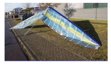
Spread the wings in steps, since the spreader bar has limited float.
