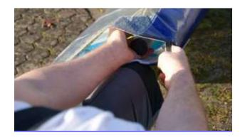
Then pull the wide, black, inside loop at the end of the sail leading edge over the end-cap of the rear leading-edge tube. There is an auxiliary loop, which helps to do this. Pay attention to the proper seating of the loop webbing in the grove of the plastic end-cap. Close the Velcro loop inside the sail to keep the black loop from moving out of its grove during transport.
